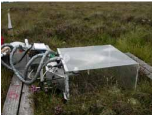
Figure 2.1. Static chamber employed to measure net ecosystem exchange (NEE).
